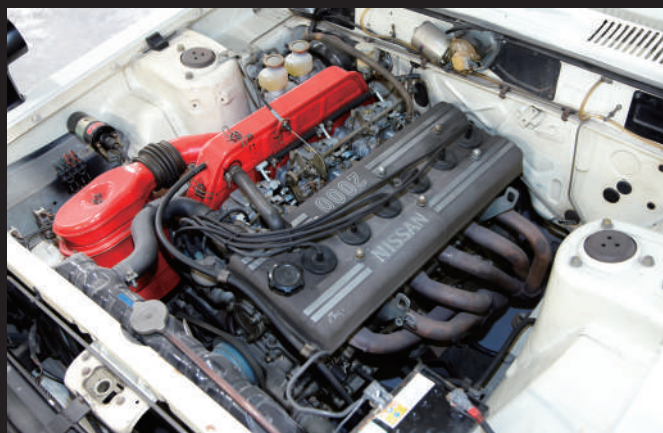
A spaciouly designed engine bay. The well-regarded S20 engine, which had been popular since the previous generation 2000GT-R, was installed.
