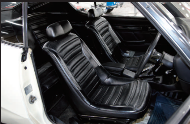
Both the driver's and passenger's seats were equipped with large bucket seats, providing stability even during cornering.
