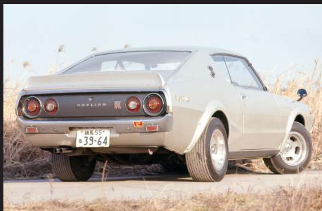
The tail lamps were transformed from square to sporty round shapes. This quad round lamp design has been carried forward in subsequent GT-R models.
