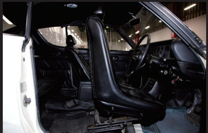
By folding the front seat forward, it was possible to access the rear seat. The passenger seat could also be operated from the driver's side.
